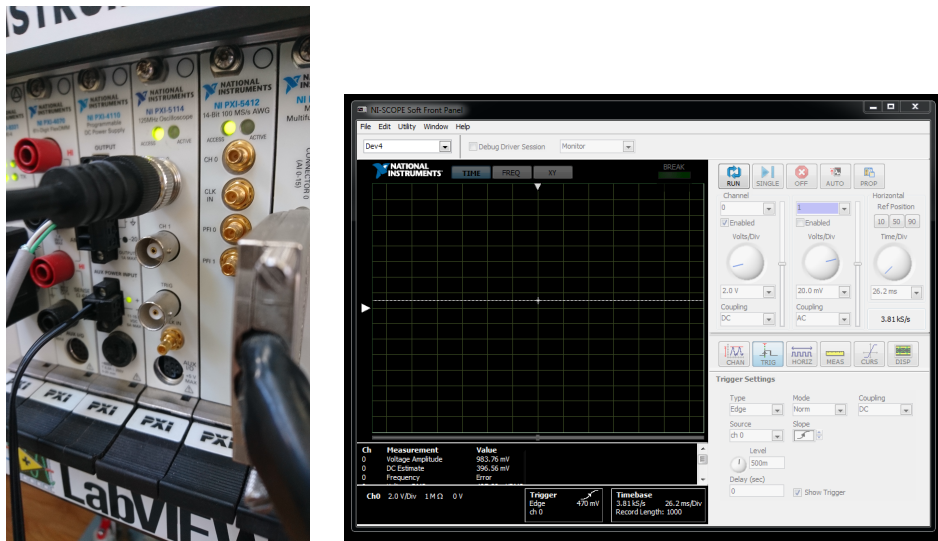
Figure 1: Left: NI PXI-5114 with coaxial probe. Right: PXI Oscilloscope Front Panel Interface
