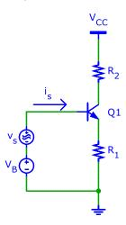
4. Design a circuit (i.e. draw the large signal circuit diagram) such that the small-signal gain  $v_0/v_s = -50$ .
