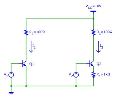
3. Derive an algebraic expression for the small-signal input resistance  $r_i = v_s/i_s$  as a function of circuit parameters  $R_1$ ,  $R_2$ ,  $V_{CC}$ ,  $I_{C1}$  and  $\beta$ .
