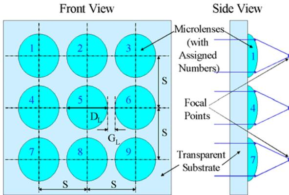
**Figure 1** Typical microlens array for Shack-Hartmann Sensor (S: Pitch between neighboring microlenses,  $G_L$ : Gap between neighboring microlenses,  $D_L$ : Diameter of microlenses, Numbers in blue: Identification numbers assigned to microlenses)
