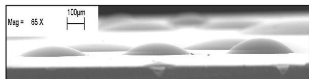
**Figure 13** Variation of microlens curvatures for 400- $\mu\text{m}$  diameter
