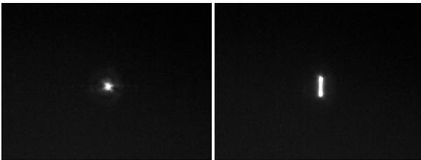
**Figure 14.** *Demonstration of focal point identification: As the microlens resonates, its focal point turns into a scanning line, and the focal point and its associated microlens can be identified. The focal length  $f$  of the microlens is 2.09mm, and the CCD imager is placed at  $9.84f$  from the lens. The focal point travels  $40\mu\text{m} \times 9.84f$  or  $0.3936\text{mm}$  on the CCD imager.*
